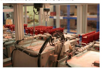
The function of the unit is to calibrate EPD's placed into the source drawer using the radioactive sources installed in the heavily shielded source modules.
