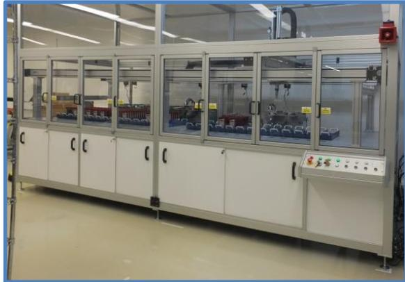
The transport system can be driven in 4 axes (x, y, z and rotational). The pick-up head attached to the Z Actuator grabs the platen holding the EPD and pick/places it within the Calibrator. The pick-up head attached to the Z Actuator grabs the platen holding the EPD and pick/places it within the Calibrator.
